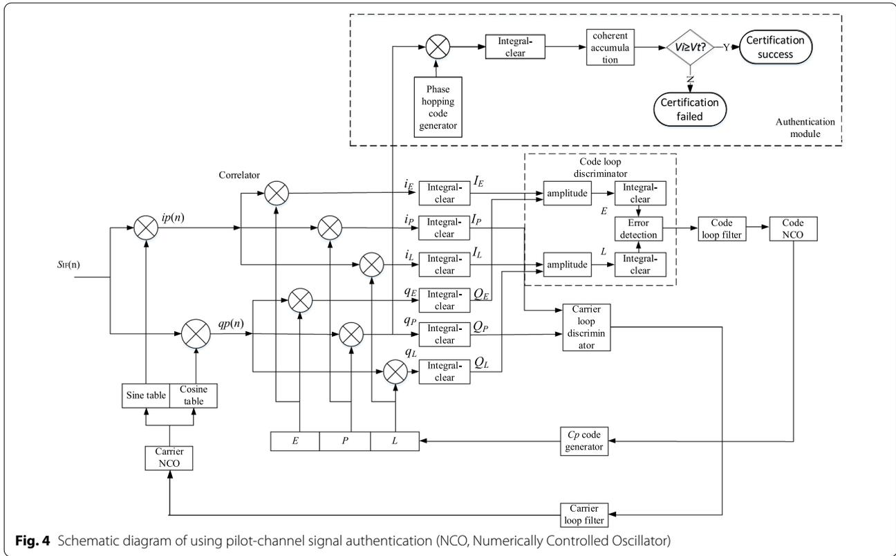
**Fig. 4** Schematic diagram of using pilot-channel signal authentication (NCO, Numerically Controlled Oscillator)
