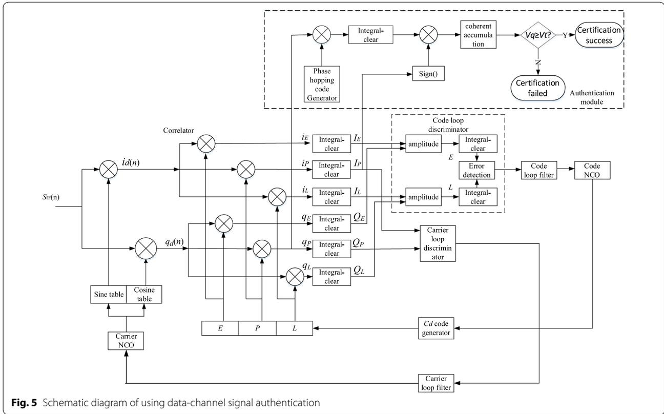
**Fig. 5** Schematic diagram of using data-channel signal authentication
