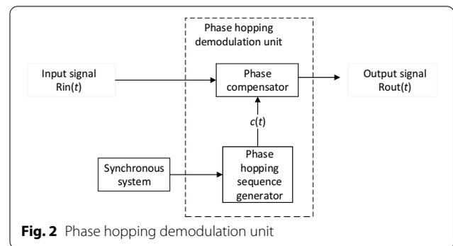
Fig. 2 Phase hopping demodulation unit
