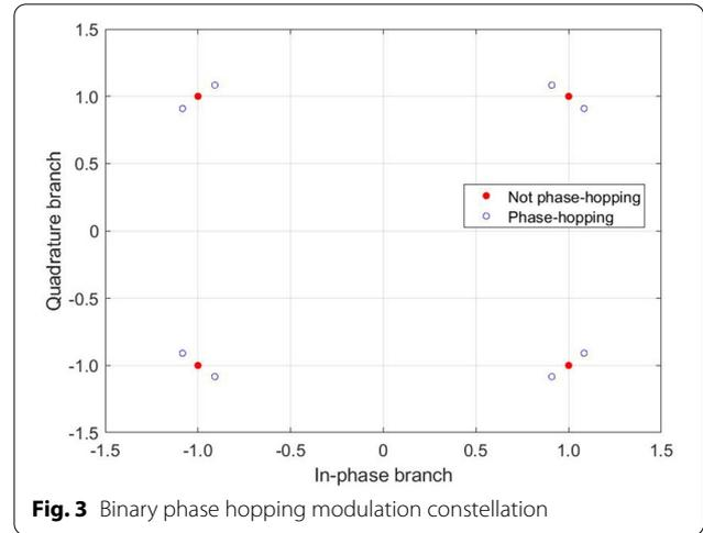
Fig. 3 Binary phase hopping modulation constellation
