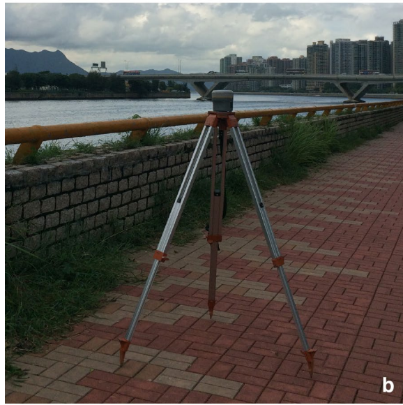
Fig. 1 a The moving station deployed beside the window in the MTR train and b the static station deployed beside the MTR train line. They were equipped with the same receiver type: the Trimble R10 receivers
