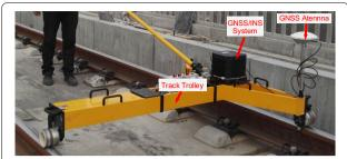
**Fig. 10** Railway track geometry measuring trolley (TGMT) based on an aided INS
