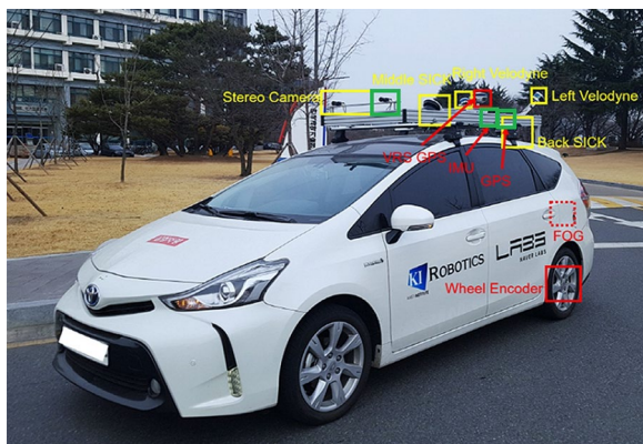
Fig. 11 Selected sensors (green boxes) in the Kaist Urban dataset Choi et al. (2018)
