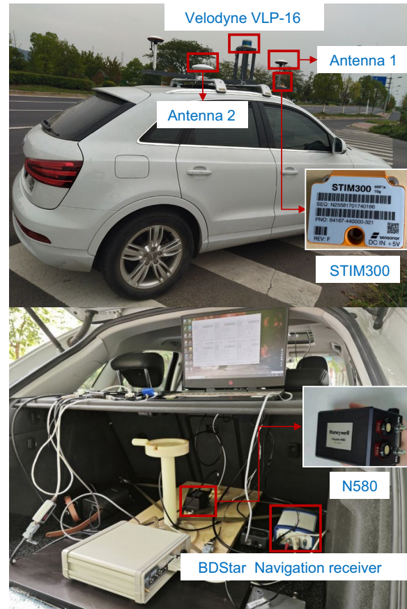
Fig. 3 The vehicle and equipment for the field test. The raw GNSS and inertial data were collected with the BDStar Navigation receiver and STIM300 IMU, respectively. One high-grade navigator, N580, was employed to provide the reference trajectory. The antenna 1 and 2 were connected with BDStar Navigation receiver and N580, respectively
