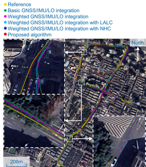
Fig. 12 Horizontal positioning results in a real map. Figure shows horizontal positioning results of these candidate algorithms in a real map, with yellow points representing the reference trajectory, green points representing the “basic GNSS/IMU/LO integration” algorithm, purplish red points representing the “weighted GNSS/IMU/LO integration” algorithm, light blue points representing the “weighted GNSS/IMU/LO integration with LALC” algorithm, dark blue points representing the “weighted GNSS/IMU/LO integration with NHC” algorithm, and red points representing the proposed algorithm, respectively
